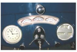
This instrument group mounted on the dashboard of the Stage. The clock is on the left, the speedometer on the right and the oil pressure, amperes and fuel pressure gauges in the top center. The ignition switch, headlight switch and ignition key are located in the bottom center.
